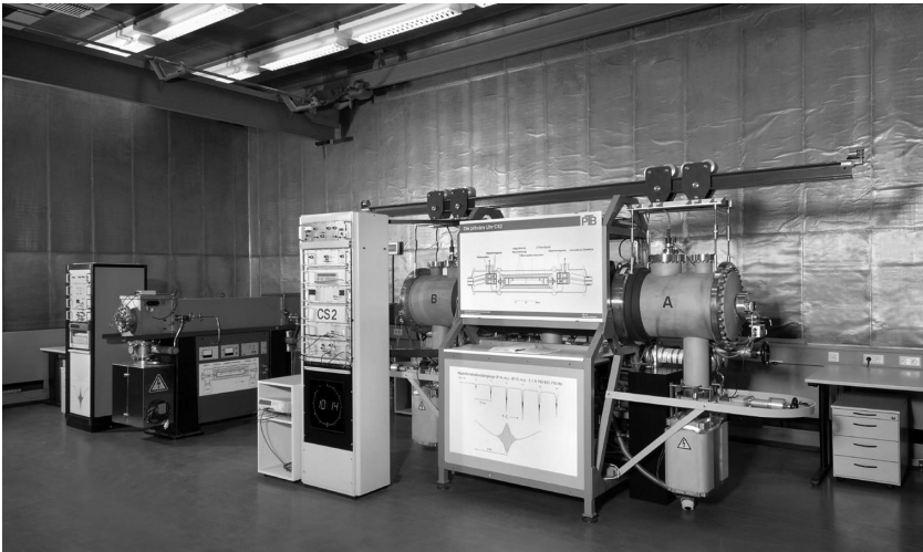
FIGURE 1.10 PTB's CS 1 and 2 developed and improved over several decades. At the time of writing the units are still used as primary frequency standards providing input to the BIPM for maintaining atomic timescale. (Courtesy of PTB, Germany.)
