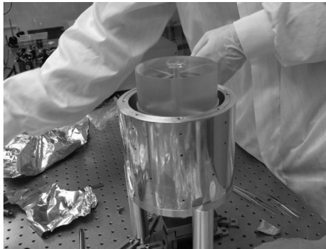
FIGURE 2.10 Photograph of the ultra-stable optical cavity used at LNE-SYRTE before final assembly. (Courtesy of SYRTE, France.)
