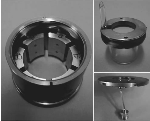
FIGURE 1.E.2 Photograph of the magnetron cavity implemented and used in an optically pumped Rb frequency standard. (Reproduced with permission from Stefanucci, C. et al., Rev. Sci. Instr. , 83, 104706, 2012. Copyright 2012 by the American Institute of Physics.)
