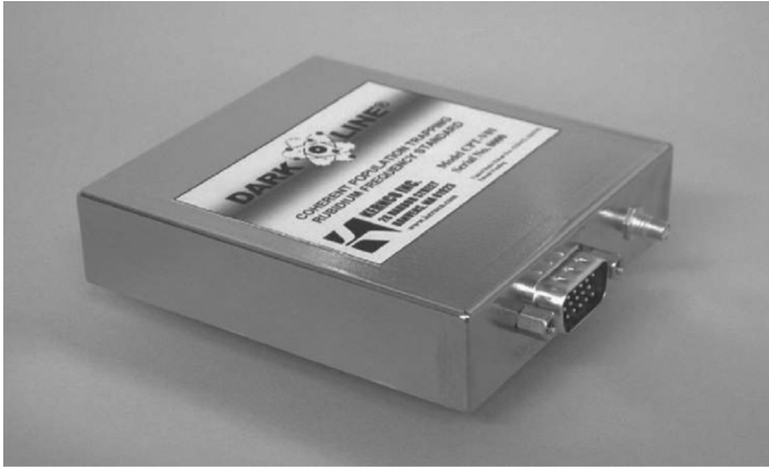
FIGURE 3.47 Commercial passive Rb frequency standard based on CPT. The system is totally autonomous, using a digital electronics approach for accomplishing the wavelength and frequency lock of the laser and microwave source to the atomic resonances. Its volume is of the order of 125 \text{ cm}^3 . (Reproduced with permission from Vanier, J. et al., IEEE Trans. Instrum. Meas. , 54, 2531, 2005. Copyright 2005 IEEE.)
